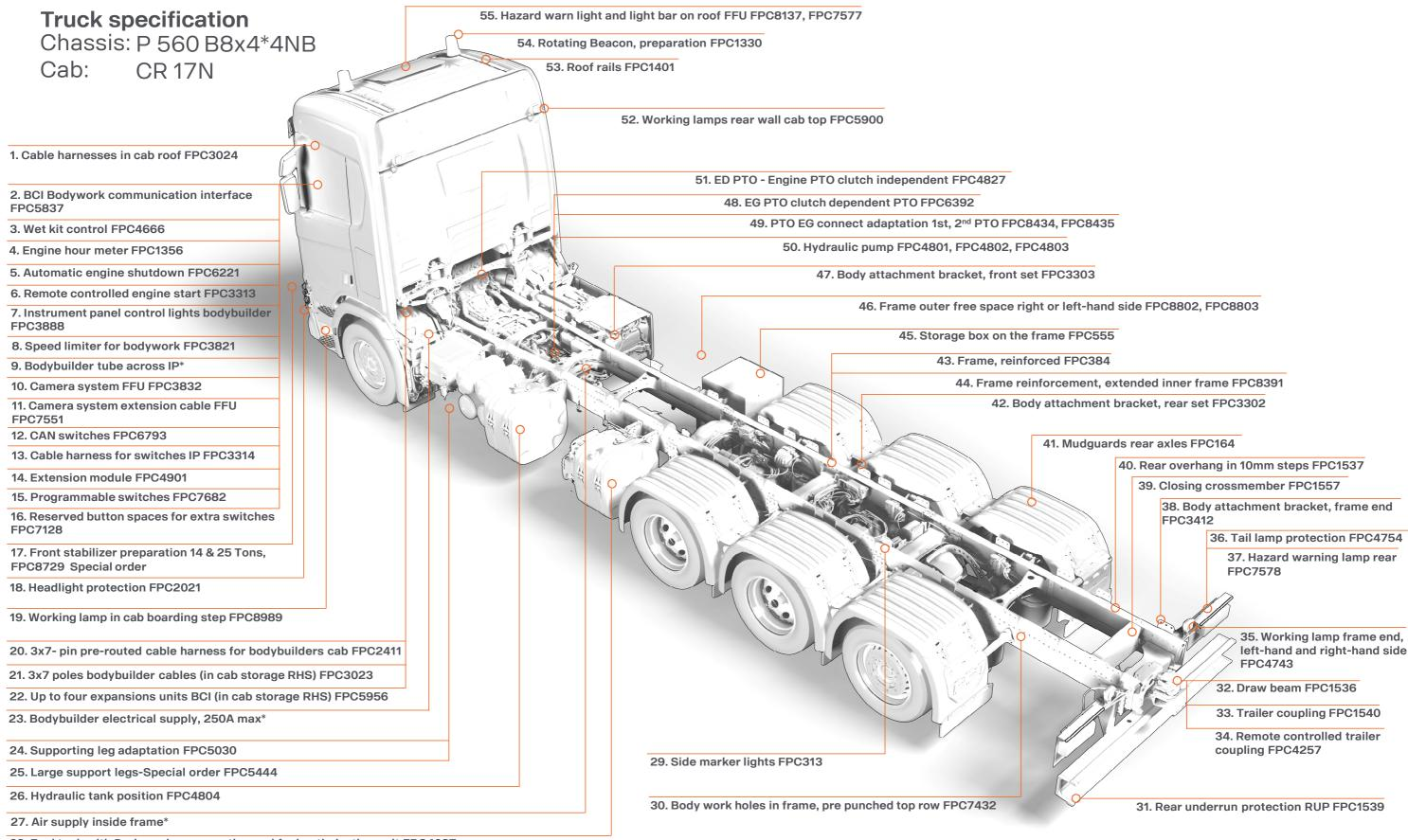
28. Fuel tank with D-shaped cross section and fuel optimization unit FPC4087
