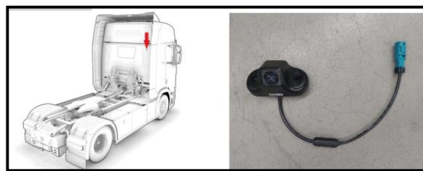
FPC11104AC, Camera connector at cab rear wall upper right corner, and camera delivered in cab
