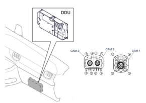
rear view camera installation or hardware. When a trailer is connected, the camera view can be automatically switched from truck to trailer camera view. This have to be setup using an external switching or prioritization interface. AHD signal format must always be used for the reverse detection camera input. If the trailer camera does not support AHD, a signal conversion is required to convert the transmitted signal from lower resolution video signal formats to AHD.
