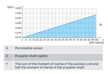
When values fall outside the permissible limit values for the propeller shaft there is a need to install an elastic coupling or similar equipment that requires a rotating force before connecting to the auxiliary equipment.
