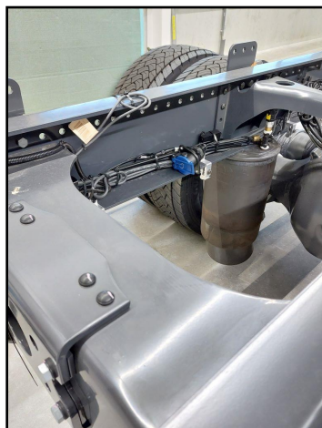
FPC11104AF: Camera trailer connector frame – Rigid chassis
