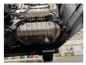
air flow is not changed or otherwise there is a risk that parts on and around the silencer, e.g. sensors, hoses, side skirt, mudguard flap and SCR-tank, can be damage by the accumulated heat from the silencer and end up in fault codes or failure on the parts.
