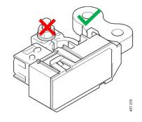
If Battery jump start interface is not available on the vehicle, battery charging or jump start connection may be connected at the batteries and then it is important to connect to the metal plate where the earth connection is connected.
