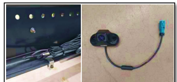
FPC11104AA: Camera connector at rear end of chassis, and AHD camera delivered in cab
