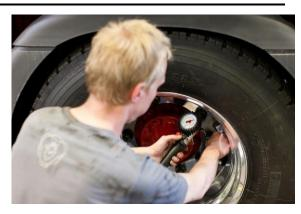
Trailer tyre pressure information up to 6 axles is transmitted by the trailer's TPM to the vehicle via EBS23 CAN and when information about the trailer tyre pressure is available it is displayed to the driver. A new sensor registration is required if a sensor is added, renewed, a complete wheel is renewed or the positions of the tyres are changed.
