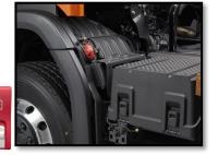
After the ignition is turned off, the system continuously monitors the battery status, if the voltage drops to 26 V or below, the function will attempt to disconnect the batteries every 6 hours and if the voltage drops to 24 V or below, the function will attempt to disconnect the batteries every 15 minutes.
